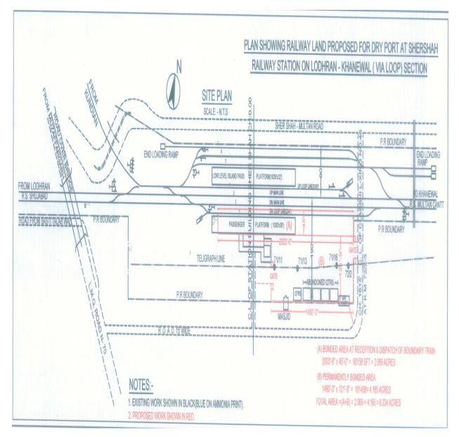
Figure 6: Proposed intermodal node at SherShah (SSH) station over the existing network of Pakistan Railways
