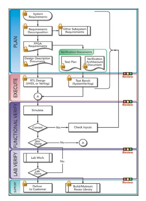
Figure 2. Typical Best Practice Electronic Design Process [11]
