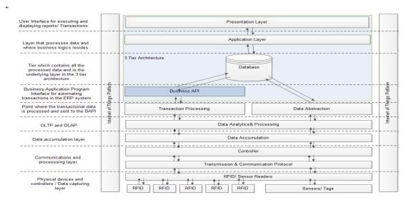
Figure 11. Conceptual Framework for Process automation through RFID and BAPPI
