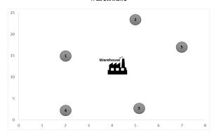
For example, the retailers are placed around the warehouse with coordinates (x, y). It is assumed that the demand rates are constant with a fleet of vehicles available in order to distribute the products.
