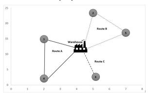
Figure 3 shows when the vehicle capacity is less compared to Figure 2, which is 30 tons. The vehicle needs to serve five retailers, but the inventory carried is not enough. In that case, the route has to extend to become three routes in order to fulfil the requirements. The vehicle has to take route A = (0-1-4-0), route B = (0-2-5-0), and route C = (0-3-0).
