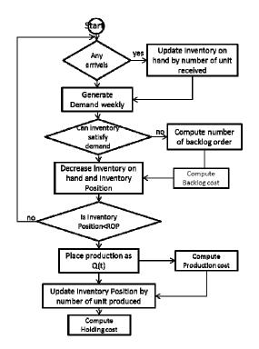
Figure 6: Simulation Flowchart for a week operation Inventory Model
