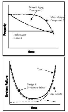
Figure 3: The predicted result of material aging against total defects output (Source: Adapted from work of Salzbrenner, n.d.)
